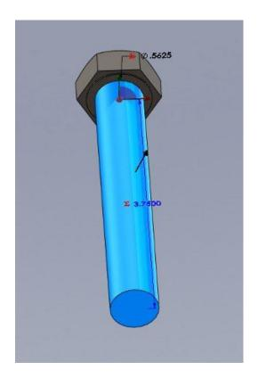
7. Apply the Bottom Chamfer feature using the derived values given to you for your design.
