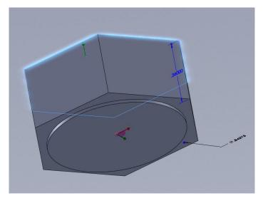
Create the Head Chamfer Cut guided by the information provided in the table above.
