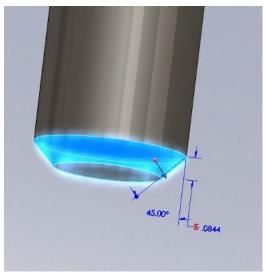
8. The final steps involve a Swept Cut feature involving a helix path and a specifically designed sketch for the cut profile. For the helix you need to sketch a circle as a parent for the Helix Feature. Select the bottom face of the Bolt Shank, start a sketch, select the outside circular edge of the shank and apply the Convert Entities sketch entity. This will project the circular edge of the Bolt Shank onto your sketch.
